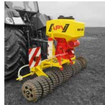
In order to ensure the contact between the seeds and the soil and to improve the germination of the seeds, the Grassland Rollers are extremely versatile. Rollers are available as Cambridge or toothed ring variation. Our seeders (Multi-Metering System and Pneumatic Seeder) can be mounted optimally for reseeding and new grass seeding.
