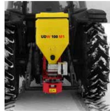
The Universal Dispensers have a metering unit made of stainless steel and are suitable for the application of salt and grit and mixtures thereof. The exact metering by means of a seeding shaft makes them a reliable working tool for use in professional winter service.
