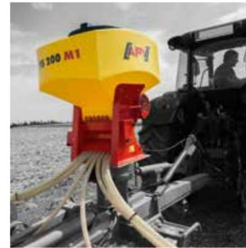
The Pneumatic Seeder covers almost all applications in the modern farming. A seeding shaft ensures precise metering. There are several hopper sizes available. The seeding close to the ground via hoses and dispersion plates promises an exact placement of your catch crops, nurse crops, grass reseeding and much more. You choose one of our control boxes individually, suitable to your requirements and needs.
