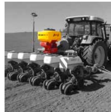
In addition to all the advantages of the Pneumatic Seeders (see above), these models are corrosion-resistant and thereby also fertilizer resistant. There are several hopper sizes available. The fertilizer edition is applicable for the application of fertilizers, micro granules as well as crop protection granules.
