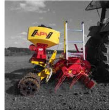
The Grassland Combi is most appropriate for reseeding in hilly terrain. Due to the great advantage that the machine can be driven both as a rear machine and separately (harrow in front, roller in the rear), it is individually adaptable to your business. The power requirement of the tractor is rather low.
