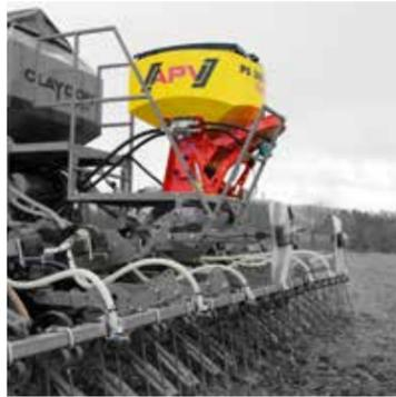
The "TWIN-PS" has a centrally divided hopper. Two various seeds, fertilisers or granules can be metered individually and independently of one another. By this means, you sort out the problems of different sizes of seeds, application rates and seeding depths.
