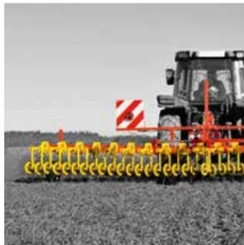
The Rotary Hoe is ideal for breaking the encrustation. The rotating hoe rings bury or uproot the weeds, promote the tillering and introduce oxygen into the soil. Due to the rotating rings, the tines remain free of plant and soil material. The chopping rings are variably adjustable from 0 to 30 degrees and thus guarantee an ideal work result.
