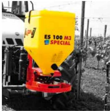
We recommend the Mini Spreader and the Single Disc Spreader Classic for small to medium working widths. The Single Disc Spreader Special achieves the best lateral distribution grade valuation (CV 9,4 % at 27 m). The spreading of slug pellets up to 28 m is possible. This model can be equipped with a sensor for the slider motor.
