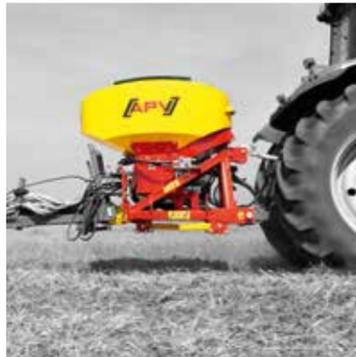
The Implement Carrier simplifies the combination of our Pneumatic Seeders with trailed cultivation implements. The seeder is installed on the Implement Carrier, only the hoses and dispersion plates are mounted on the cultivation implement. The result is an optimal weight swift: You shift the weight from the implement's frame to the rear axle of the tractor.
