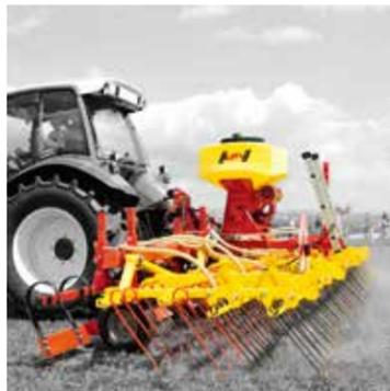
The Grassland Harrow works intensively and reliably with a unique combination of 10 mm and 8 mm tines. The aggressiveness of the working process is individually adjustable. Despite the rather low power requirement of the tractor you still achieve a high area performance. Levelling, harrowing and reseeding - all in one pass.
