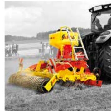
The Grassland Pro Harrow meets today's requirements of intensive maintenance of meadows in professional farming and contracting. Due to the unique combination of strong 12 mm tines and 8 mm tines, the grass sward is tilled to the optimum. The trailing roller assures the reconsolidation and soil contact with the seeds.
