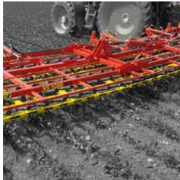
The Tined Weeder Pro VS adjusts with its unique tine spring system to the soil and protects the culture plant at the highest level. The tine pressure remains constant at different tine levels. As a result, crops planted on ridges, such as the potato, can also be harrowed. The tine pressure is identical on the ridge crown, ridge flanks and in the furrow.
