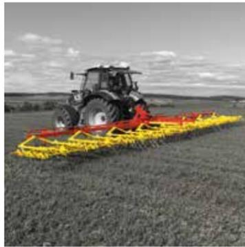
The main focus of the Tined Weeder AS is on combating unwanted weeds. While the tines sweep over the soil, the weeds, which are already in threads or germ stage, are mostly buried, pulled out and deposited on the soil surface. This means that approximately 90 % of the weed germs are decimated.
